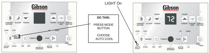
Note: In this mode when the room temperature is reached the compressor will shut off and after a few minutes the fan will switch to the lowest setting, (if a higher setting has been originally selected). When the compressor switches back to the cooling mode, then the fan speed will return to the original setting.
